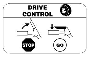
The drive control is located on the right handle. Squeeze the control grip against the handle to engage the wheel drive. Release to stop.
